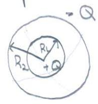
$$C = \frac{R_1 R_2}{R_2 - R_1} \quad \left. \vphantom{C} \right\} \text{Caso concêntricos}$$
