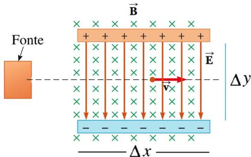
$$\Delta y = r - \sqrt{r^2 - \Delta x^2} = \frac{mv}{qB} - \sqrt{\frac{m^2 v^2}{q^2 B^2} + \Delta x^2}$$
